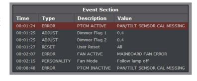
power up and the pan/tilt sensor was not calibrated (warning was listed as ACTIVE) 1 minute and 24 seconds after power up but was calibrated (warning was listed as INACTIVE) 8 minutes and 48 seconds after power up.
